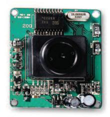
Our high performance 1/3" B/W CCD board camera with pinhole lens allows for easy concealment. Features a 3.6mm wide angle lens, 0.5 lux and 420 line resolution. Includes wiring harness for easy installation. A 12V DC power supply is required (not included)
