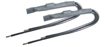
DITEK's DTK-ESS SPD (Surge Protective Device) protects electric door strikes. Electric door strikes (magnetic locks) are typically installed in metal frames, with low voltage wiring back to an access control panel, creating a vulnerable surge path. The compact ESS installs in the door frame to prevent voltage surges from getting into the control panel.
