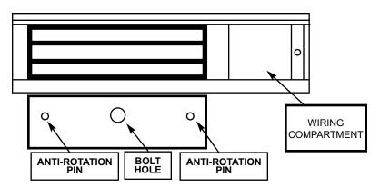
WHEN MOUNTING ARMATURE PLATE ON DOOR RUBBER WASHER MUST BE PLACED BETWEEN METAL WASHERS. DO NOT EXCESSIVLY TIGHTEN SEX BOLT. ARMATURE MUST FLOAT ON DOOR. THREAD LOCKING AGENT SHOULD BE USED.
