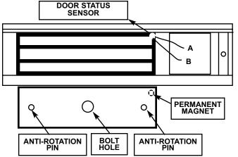
INSTALL THE MAGNET AND ARMATURE PLATE AS SHOWN. IF NOT POSITIONED AS SHOWN THE OPERATION OF THE SENSOR OUTPUT WILL BE AFFECTED.
